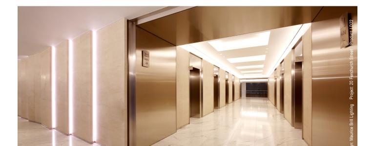
LD22 is a very small, low profile linear system. Designed to maximise the light output with a broad beam, it is ideal for coves, shelf details, recesses and highlighting architectural details. It is a 24V DC system allowing long lengths to be powered from a single driver.
